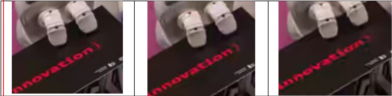
Figure 5b): Cropped section of a frame from CatRobot encoding using, from left-to-right, VVC BMS1, HEVC HM16.18, and AV1, respectively, in constant Q mode, showing decreasing subjective visual quality (see fingers, text).
