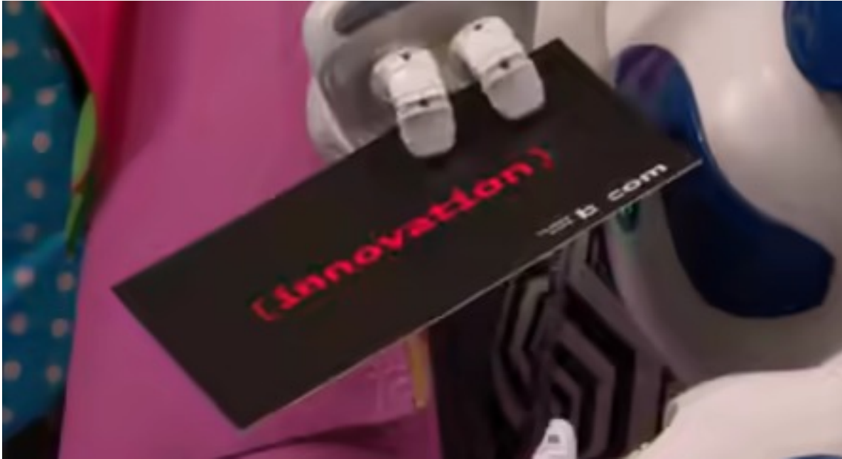
Figure 7. Cropped section of a frame from CatRobot sequence reconstructed after encoding with AV1 under target bitrate mode (VBR). Note that the subjective visual performance is now on par with HEVC.
