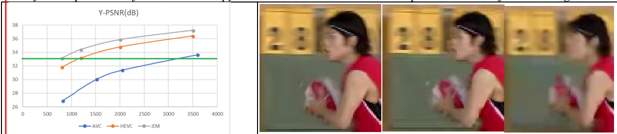
Figure 2. FastVDO example extreme low bitrate coding, with 3 codecs (AVC/HEVC/VVC draft), on a 1080p50 sequence (Basketball Drive), with (a) objective metric Y-PSNR; (b) crop visuals at 0.8 Mb/s (that is 3000:1 compression!), using VVC, HEVC, and AVC (H.266/5/4) L to R. (a) Hor. Line suggests that as of now, 0.8 Mb/s VVC ~ 1.2 Mb/s HEVC ~ 3.2 Mb/s AVC (VVC=1.33X HEVC = 4X AVC in coding efficiency).
